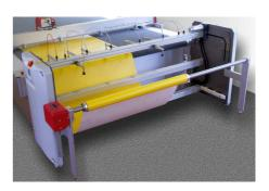
The machines also can be converted to Production Line Cutters (PLC) with integrated loading and/or unloading table.
